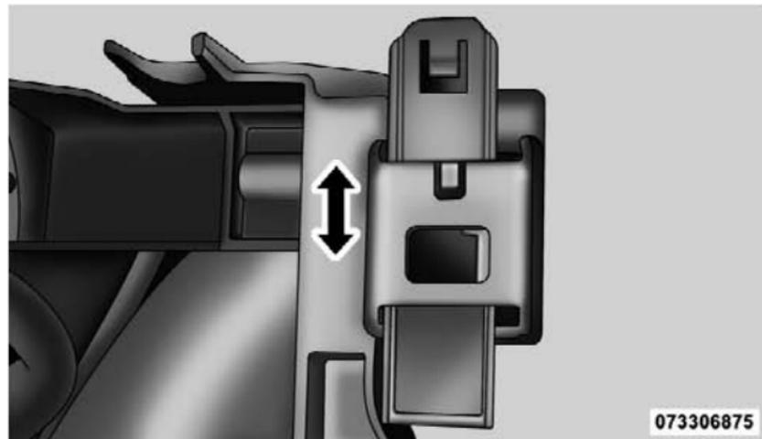
9. Remove the headlamp assembly. Grasp the outboard edge of the lamp and pull it straight forward to disengage the ball stud from the plastic grommet.
