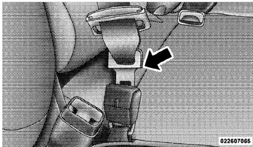
Inserting Latch Plate
