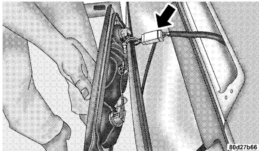
3. Turn the desired bulb socket  $\frac{1}{4}$  turn and remove the socket and bulb from housing.
