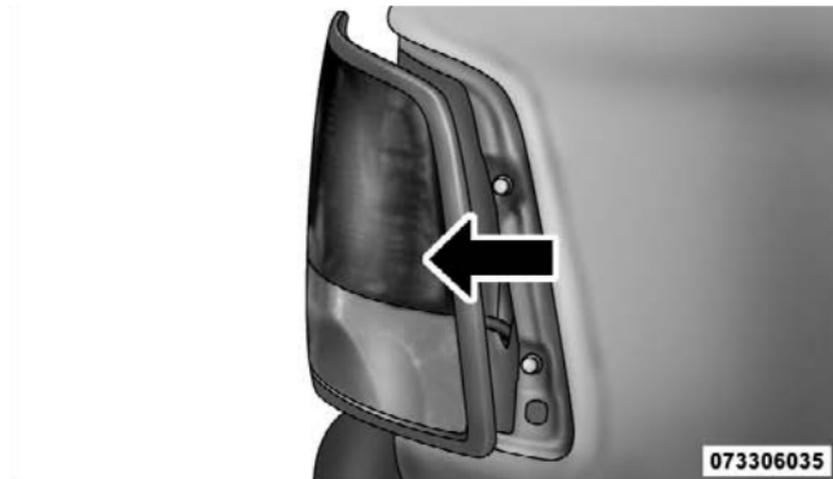
3. Disconnect the wiring harness connector from the bulb socket.
